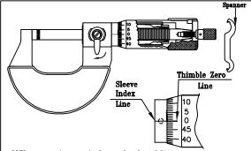
If The zero setting error is about or less than ±0.01 mm.
