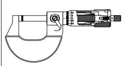
Reassemble the Knurl ring, thimble cap & speeder knob.
