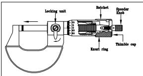
Clean the Measuring faces thoroughly. Use RATCHET to flush or bridge the measuring faces with each other (or with the faces of setting gauge for above 25 mm) & lock the SPINDLE by LOCKING UNIT & read the value.
